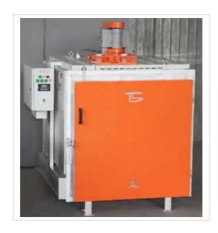
Furnace for heat treatment of parts during strain gages bonding, as well as other heat treatment works.
