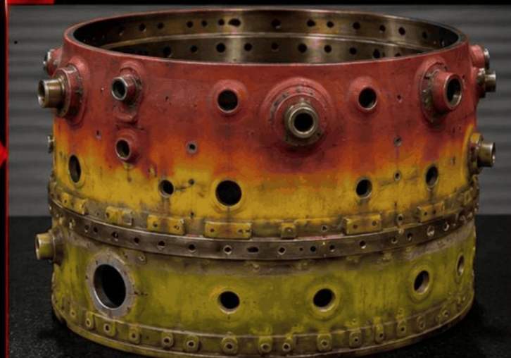
Post-test colour map used to identify peak surface temperatures
